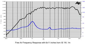
ree Air Frequency Response with 6x11 inches horn @ 1W, 1m Impedance (without horn)
